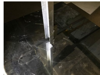
Figure 20: 460mm (920mmΦ) horizontal movement was recorded Source: Nikken Sekkei Archits. & Engrs
