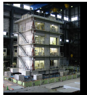
Figure 16: Life size mockup hospital building on shaking table Source: National Research Institute for Earth Science and Disaster Resilience, Japan
